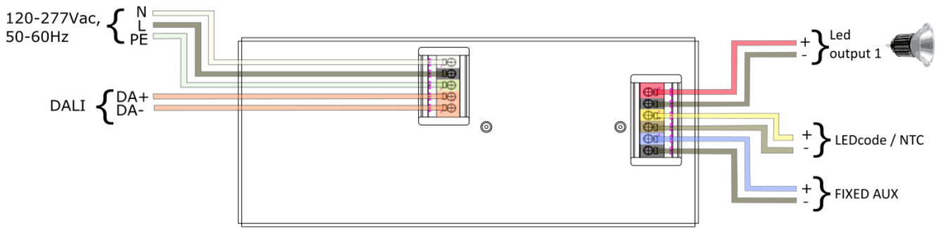
Figure x – Wiring for the EC75B-M1A0D and SL75B-M1A0D
