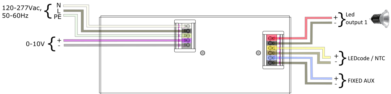
Figure x – Wiring for the EC75B-M1A0A and SL75B-M1A0A
