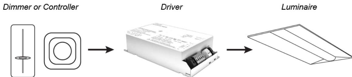
Figure 1 – Typical LED dimming system
